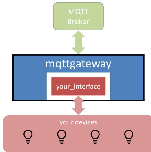
mqttgateway is a python framework to build consistent gateways to MQTT networks.
